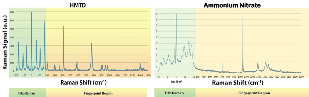
Ondax's patented<sup>2</sup> **THz-Raman<sup>®</sup> Spectroscopy Systems** extend the range of traditional Raman spectroscopy into the terahertz/low-frequency regime, exploring the same range of energy transitions as terahertz spectroscopy – without limiting the ability to measure the fingerprint region. This enables **simultaneous analysis** of both molecular structure and chemical composition for advanced materials characterization.
