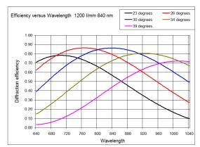
Wavelength tuning allows a single VPH grating to be used at multiple AOIs to span a larger region of the spectrum, reducing the cost and complexity of your broadband spectrographic system design.
