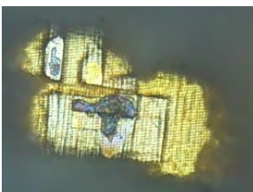
Remove EPOXY on surface by 266 nm
