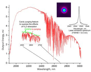
Typical Tuning Curve of CLT-5 Laser
